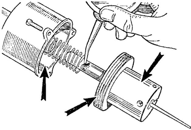
Fig. 6: Oil only piston rod. Surfaces at arrows must be clean and oil-free.
