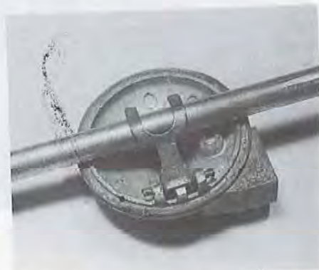
8.6 Checking the float level setting with a 0.44 in (11.0 mm) diameter twist drill
