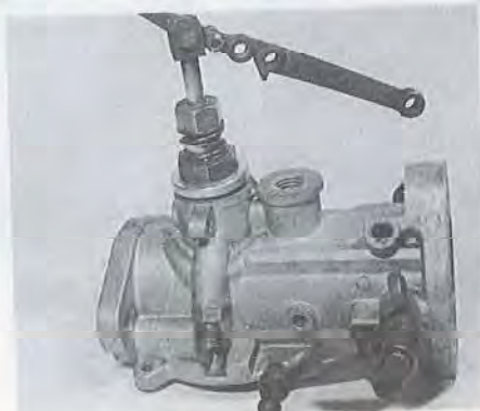
8.2B Refitting the jet assembly
