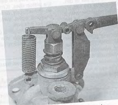
7.6A Jet control lever and return spring
