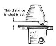
or level with the top of the jet. Now measure the gap of the float to the lid, for future reference. On my carbies I have found this to be 7/16". When the float has been adjusted replace the lid on the float bowl.
