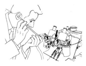
The third method is to use a device called a Unisync, which is basically an air flow meter.
