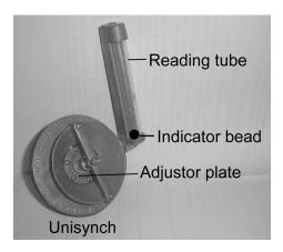
How this device works is that you tightly hold it against the input throat of one of the carbies, adjust the "adjustor" plate until the indicator bead is about half way up the reading tube. Then you place it against the other carbie and adjust the idle screw until the bead is in the same place, up the tube, as on the first carbie. Repeat until both carbies remain at the same setting.
