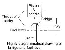
The level is adjusted in one of two ways. With the earlier and the latest floats the metal hinge is bent up or down to get the desired fuel level. With the all plastic floats washers are added or subtracted from under the needle valve to raise or lower the fuel level, more washers give a lower fuel level. When bending the hinge, be careful that the float doesn't hit
