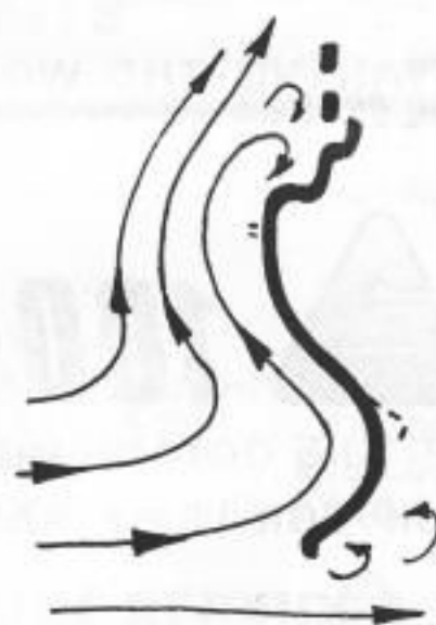
Poor air dam profile (power-consuming flow reversal and turbulence)
